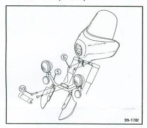
26. Check the position of the Passing Lamps and Turn Signals. If necessary, remove the rings and Passing Lamp bulbs, then loosen the Special Bolts (9) and adjust the positioning. Tighten the Bolts and then reinstall the bulbs and rings.
