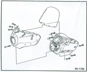
5. Remove the chrome cover from the turn signal mount. Unscrew the two Allen bolts holding the turn-signal mounting bar, then unplug the turn signal wires (noting the wire color codes for each side).
