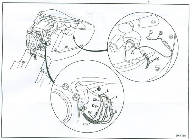
21. Using the Wire Connector ③ provided, splice the Red wire ⓓ from the Passing Lamp Harness to the motorcycle's wiring harness. Choose the correct wire for the proper lighting according to your state regulations as follows:
