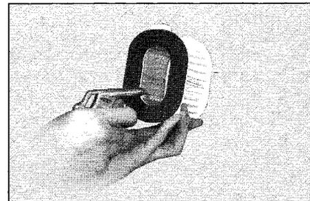
5. Tap the air filter lightly to remove most of the dust and dirt and blow out the remaining dirt with compressed air as shown. If the air filter is damaged, replace it.
