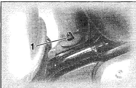
1. Rear shock absorber air valve cap
